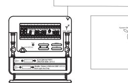
Transmitter thermostat is powered by 4 x AAA Alkaline, 2 batteries to power the thermostat, another 2 designed to provide power to Blue-backlit/Red-Indicator.
