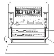
Flip to open the flap on front plastic housing. Upper compartment 2 x 1.5V AAA for powering transmitter.
